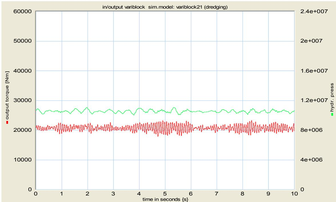
Figure 7: 20-Sim simulation output, torque in intermediate shaft and hydraulic pressure.
