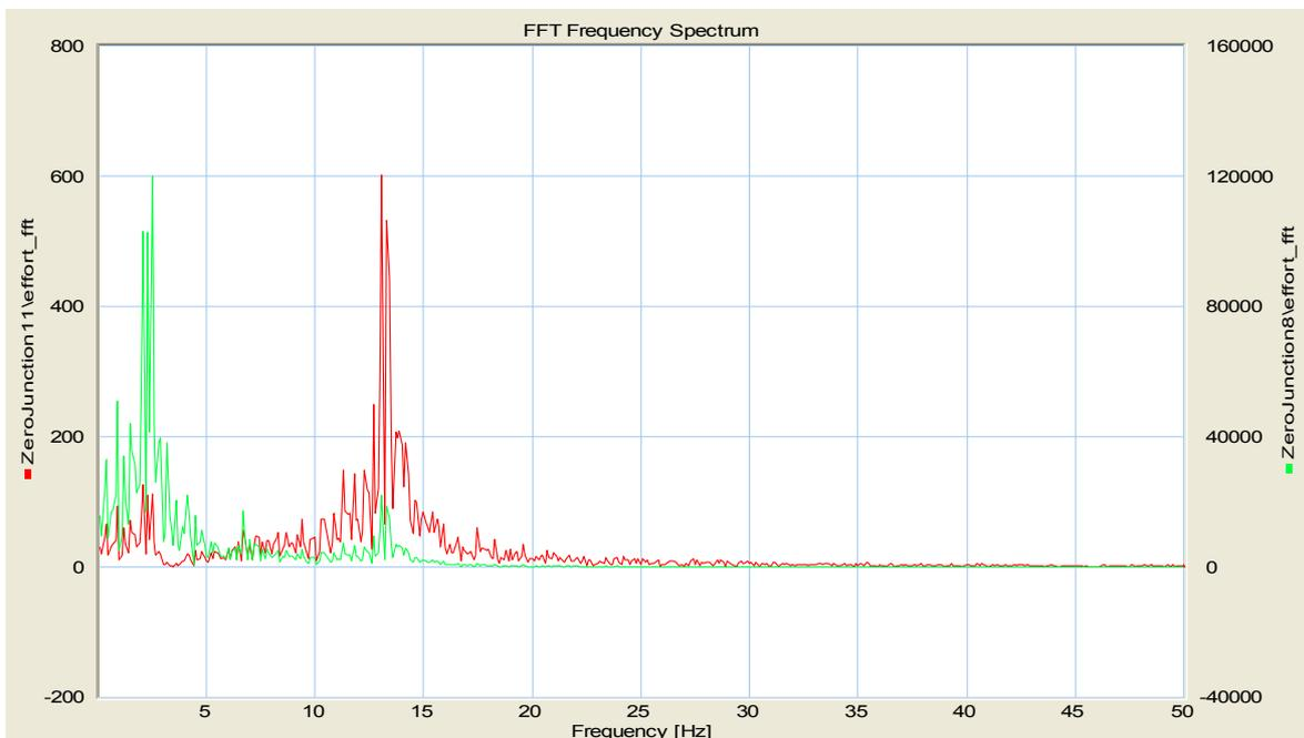
Figure 8: FFT of the simulation output of fig 7.
