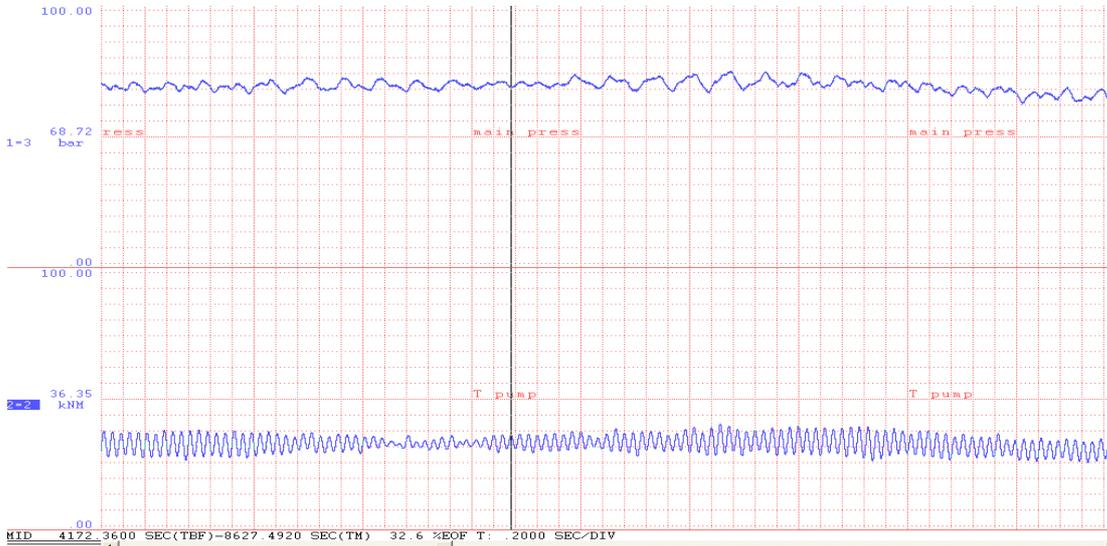
Figure 5: Measured hydraulic pressure and dredge pump shaft torque during dredging.
