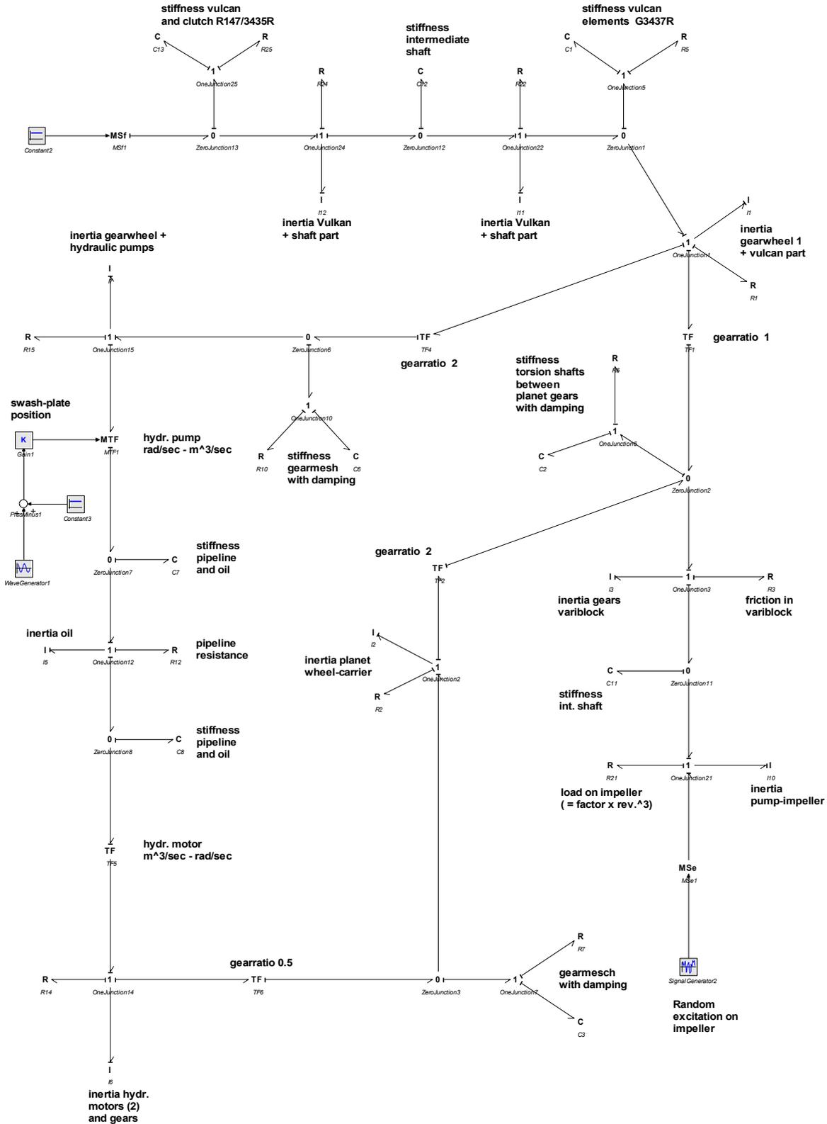
Figure 4: The bond graph model of the dredge pump drive entered in 20-sim.
