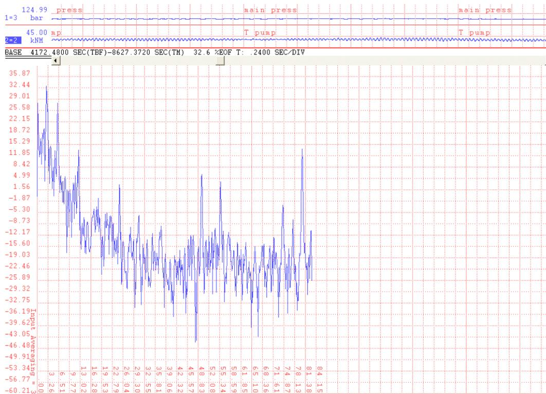
Figure 6: FFT analysis of the measured hydraulic pressure from figure 5.
