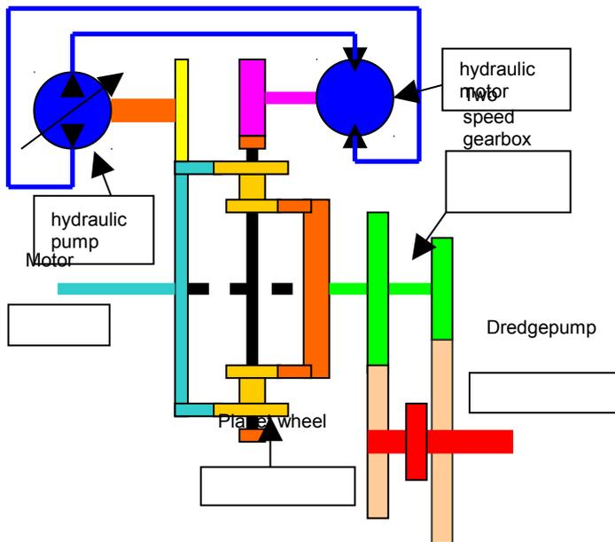
Figure 3: Physical system of the dredge pump drive.
