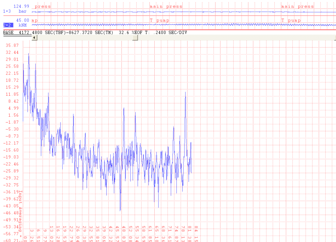
Figure 4: FFT analysis of the measured hydraulic pressure from figure 4.
