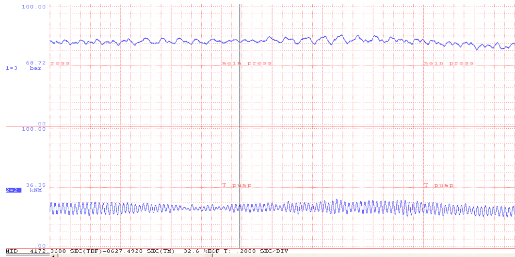
Figure 5: Measured pressure and dredge pump shaft torque during dredging.
